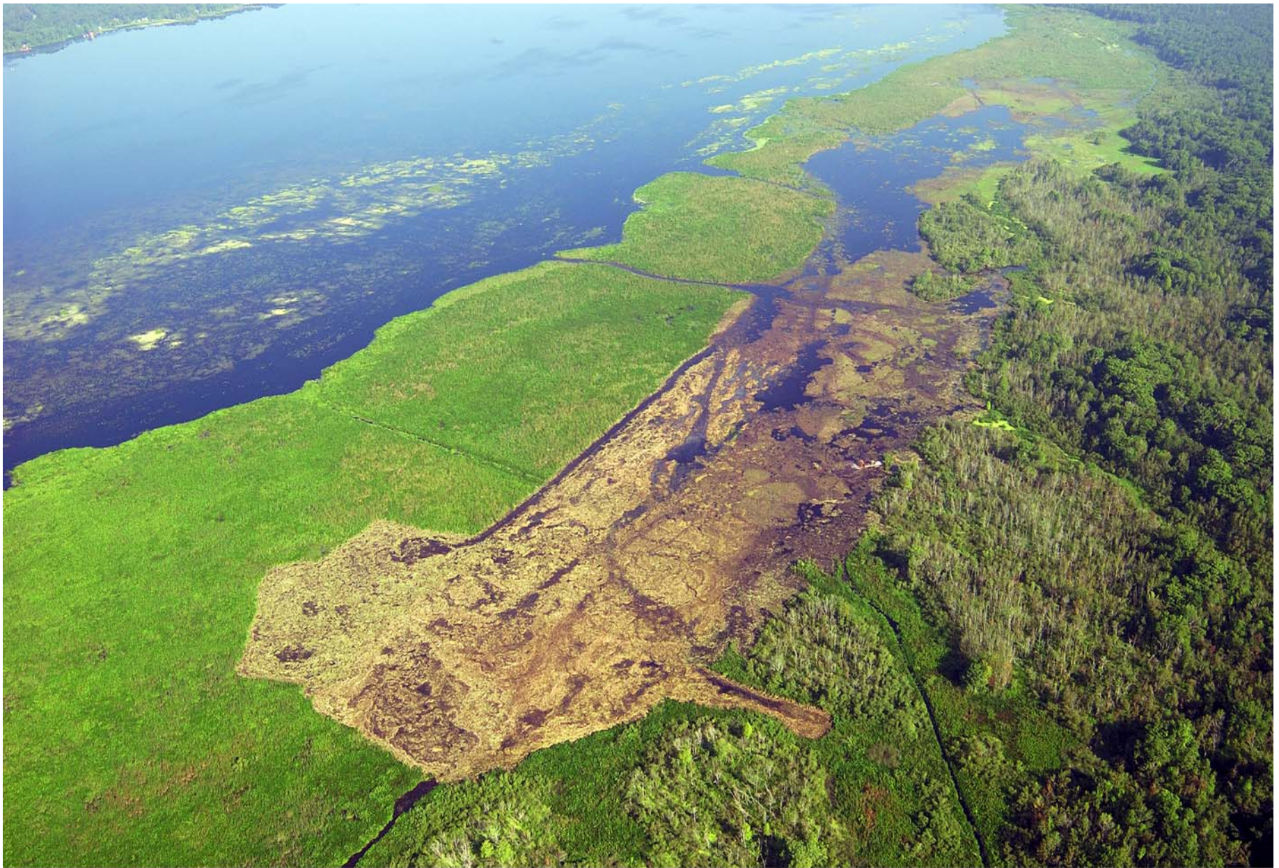
Figure 7 – Area along the eastern shoreline immediately north of the Coleman Landing channel where the dense emergent vegetation and tussocks have been chopped up by the “Cookie Cutter” machine
